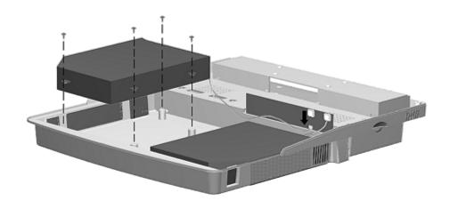
Figure 7-31. Removing the Speaker Assemblies
